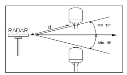
1.5.2.2 The FleetBroadband antenna may also interfere with other radio systems. Especially other Inmarsat systems and EPFS receivers with poor frequency discrimination are vulnerable to the radiation generated by the FleetBroadband antennas.
